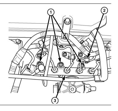
12. Position proper fuel line to proper injector on engine, tighten fittings hand tight at both ends of the line.
