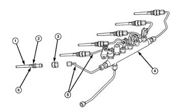
13. A connector retainer (nut, 3, outlined in red) is used on each connector tube. Remove this nut(s) by unthreading from cylinder head.
