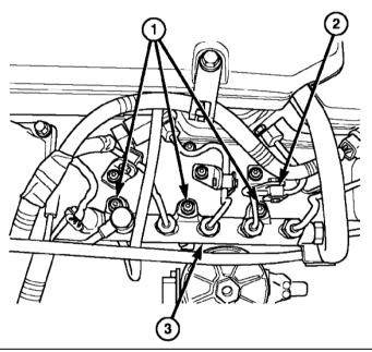
16. Tilt metal bracket upwards and tighten 2 bolts at the rear of cylinder head to **43 N.m. (32 ft. Ibs.)**
